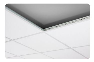
Parafon Hygiene is a highly durable acoustic tile developed for suspended ceilings in rooms with stringent requirements for good hygiene and cleaning. The surface is a white reinforced glass-fibre felt that is particularly scratch resistant and tolerates high and low-pressure washing and cleaning with disinfectants.
