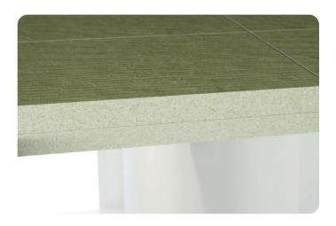
Parafon Bass is a supplementary sound absorber that is placed above the visible acoustic ceiling in order to provide absorption in the plenum for different purposes. Parafon Bass is manufactured in non-combustible rockwool with a thin glass-fibre felt on the front and back, and thin spray painted edges. The product is not visible after installation and imperfections and colour variations will occur.
