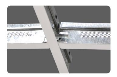
The Teetanium T15 MX15 is a galvanized steel click system with high torsional strength from the manufacturer Cipriani. The main runner profile has a fire break feature and the cross tee has an extra long lip facilitating the installation. Connection is made with an audible click.
