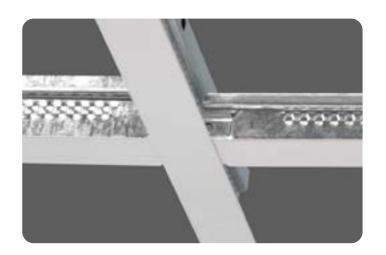
The Teetanium LG24 is a T-24 galvanized steel suspension system with high torsional strength from the manufacturer Cipriani. The main runner profile has a fire break feature and the cross tee has an extra long lip facilitating the installation. Connection is made with an audible click.
